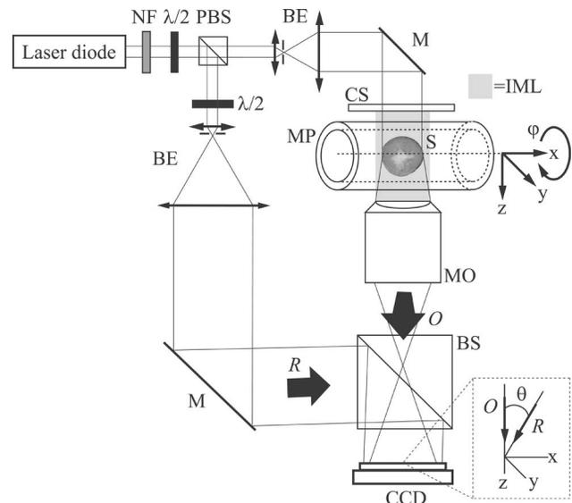
Fig. 1. Holographic microscope for transmission imaging: NF, neutral-density filter; PBS, polarizing beam splitter; BE, beam expander with spatial filter;  $\lambda/2$ , half-wave plate; MO, microscope objective; M, mirror; BS, beam splitter; O, object wave; R, reference wave; MP, micropipette; S, specimen; IML, index matching liquid. Inset: detail showing the off-axis geometry at the incidence on the CCD.
