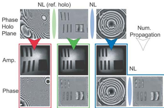
**Figure 3.** Complete numerical compensation for image distortion and phase aberration induced by a lens ball used as microscope objective. Red arrow: image reconstruction without compensation; green arrow: image corrected with the reference hologram correction method; blue arrow: manual compensation for residual image distortion. NL: numerical lens.
