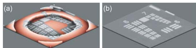
**Figure 2.** The computed aberration coefficients on the assumed flat areas, red in (a), define the numerical lens that provides the unaberrated topography (b).
