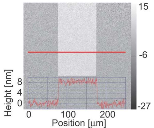
**Figure 4.** (a) Topography and extracted profile of a  $8.9 \pm 0.5\text{nm}$  calibrated high step obtained with a 20x microscope objective. The digital optics (here reference hologram) allow subnanometer resolution.
