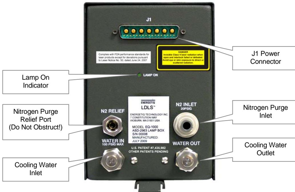
**Figure 7: Lamp Unit Rear Panel**
