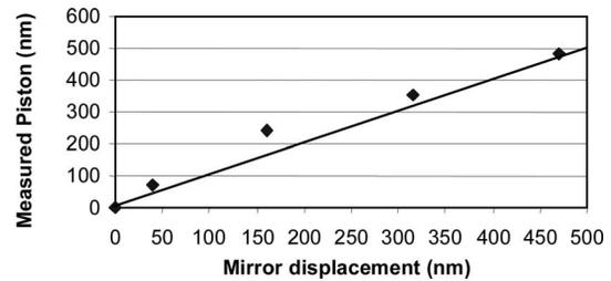
Fig. 5. Amplitude of  $P(x)$  is equal to the piston with an average error and a sensitivity of 40 nm.
