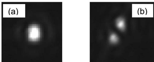
Fig. 3. (a) A single focal spot is observed for a piston value of 0 while (b) a symmetrically split spot is observed for a piston value of  $\pi$ .
