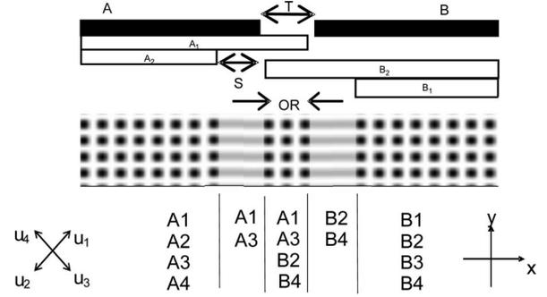
Fig. 1. Replication of independent beams  $A$  and  $B$ , separated by a physical gap whose thickness is  $T$ ; on the top by a 2-wave shearing interferometer, on the bottom schematic interference pattern of 4-wave replicas.
