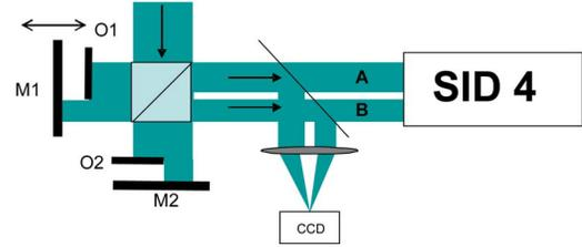
Fig. 2. (Color online) Mirrors  $M1$  and  $M2$ , and beam blocks  $O1$  and  $O2$  deliver two independent subbeams  $A$  and  $B$  separated by a physical gap; their relative piston misalignment is analyzed by a far-field sensor and a QWLSI.
