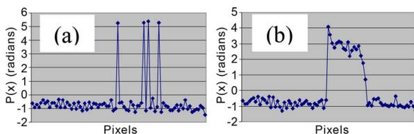
Fig. 4. (Color online)  $P(x)$  is a top hat function, whose amplitude is equal to the piston. (a) For a piston equal to zero,  $P(x)$  beats between 0 and  $2\pi$  (optically equivalent). (b) Example for a piston close to  $2\pi$ .
