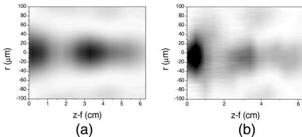
Fig. 6. Focal-spot regions of a beam modulated by a hologram producing a line of 6.3 cm. (a) Fresnel diffraction simulation. (b) Experiment: The intensity damping is due to the fact that the experimental beam was Gaussian.
