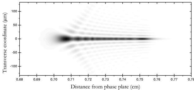
Fig. 4. Fresnel-diffraction-simulated focal region of the beam, focused with a phase plate designed to create a focal line. The line gets thinner and thinner at its end and is less than 50% of the diffraction limit for the same aperture in the near field.
