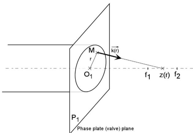
Fig. 3. Ray-tracing notation. A ray issuing from point M at radial coordinate  $r$  will intersect the optical axis at  $z(r)$ , located between  $f_1$  and  $f_2$ , the extreme focus positions.
