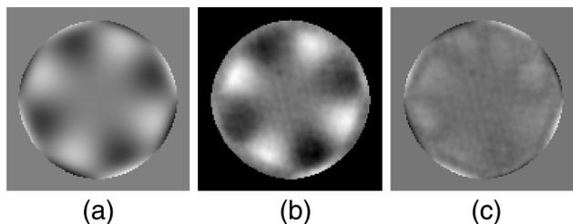
Fig. 2. Arbitrary phase-profile convergence. (a) We let the wave front coverage to  $(n = 2, m = 4)$  Zernike polynomial. (b) Measured wave front at the end of the loop. (c) Normalized error. The rms of the error is  $\lambda/76$ .
