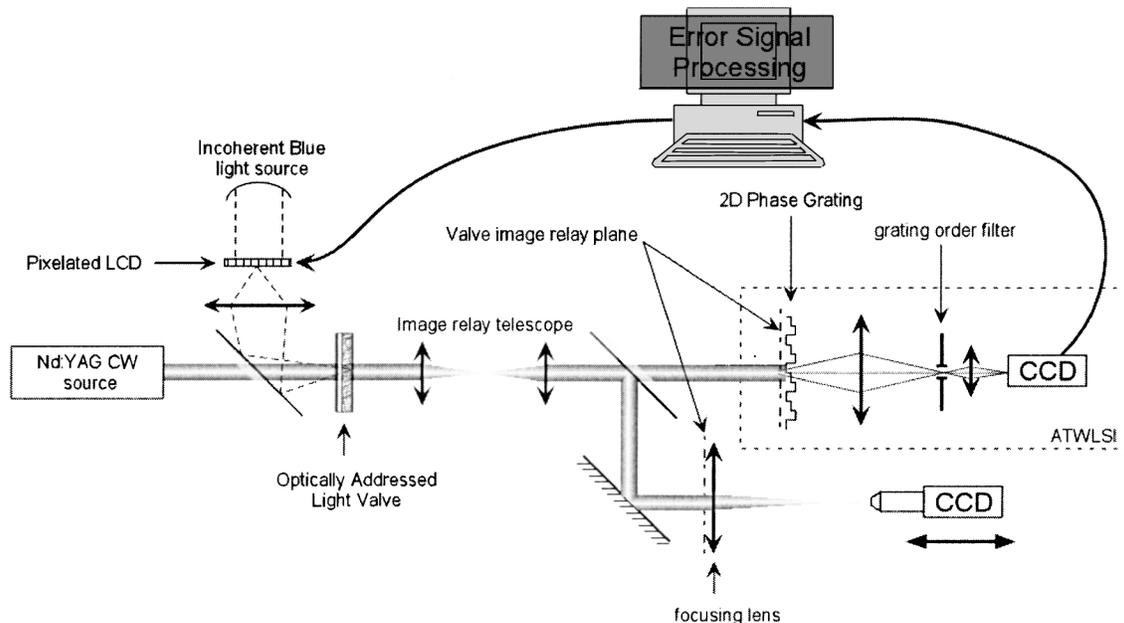
Fig. 1. Experimental setup for beam shaping. The liquid-crystal optically addressed spatial light modulator modifies the spatial phase that can be monitored by the achromatic three-wave lateral shearing interferometer (ATWLSI). The far-field pattern is imaged by a 10× microscope objective and recorded by a CCD camera. 2D, two-dimensional.
