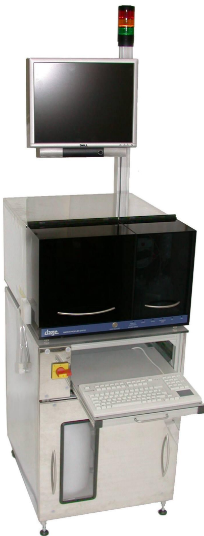
CVP21 including option FP: Footprint 60*80cm for minimum required clean room space
