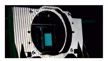
The surface of an object is illuminated with a sequence of fringe patterns. A camera observes the illuminated object and its surface shape is calculated according to the resulting displacement of the fringes. The required fringe patern can be realized with ultimate precision by HOLOEYE Liquid Crystal on Silicon (LCOS) microdisplays.
