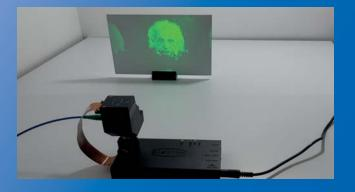
The diffractive approach with a phase SLM is fairly simple as it only requires a linearly polarized light source and the SLM itself. However, as diffraction angles are limited (dependent on pixel size of the used SLM) it might be necessary to use additional optics to magnify the output image.
