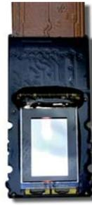
Different phase display versions can be driven with the same LUNA driver unit. Currently the LUNA series covers a versions for the visible (420-650 nm) and a version for typical telecommunication wavelength in the area of 1400 - 1700 nm (e.g. C-Band 1550 nm).
