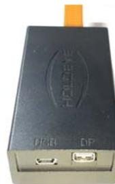
The driver features an up-to-date DisplayPort interface and an USB connector for power and advanced
