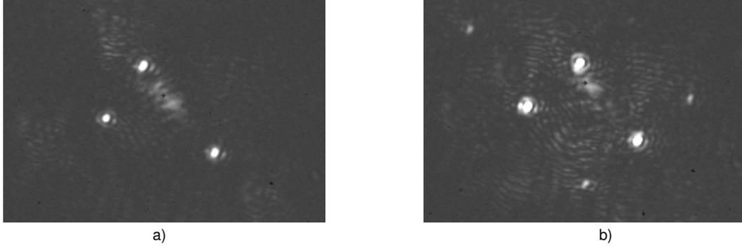
Fig. 5. Three traps produced by the “random mask” (a) and the “gratings and lenses” (b) algorithms, respectively.
