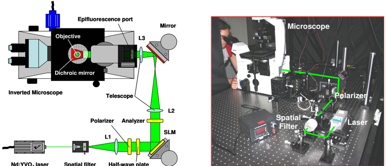
Fig. 1. Optical setup for generating holographic optical tweezers
