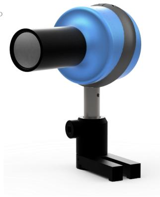
The TeraPyro sensor is a compact and highly sensitive device, based on the combination of a high-quality absorbing black coating, paired with a LiTaO3 pyroelectric crystal. The broad absorption range of the coating allows the use of this sensor over a large spectral range (from 0.1 to 30 THz). The high sensitivity and low NEP offer no compromise on performances. The integrated, pre-aligned, high quality THz optics based on AR coated Si-lenses ensures
